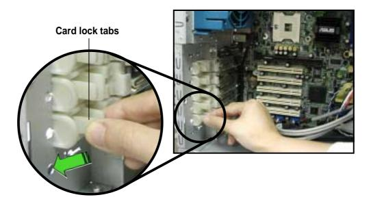
Carefully install an expansion card making sure that it is properly seated on the slot.
